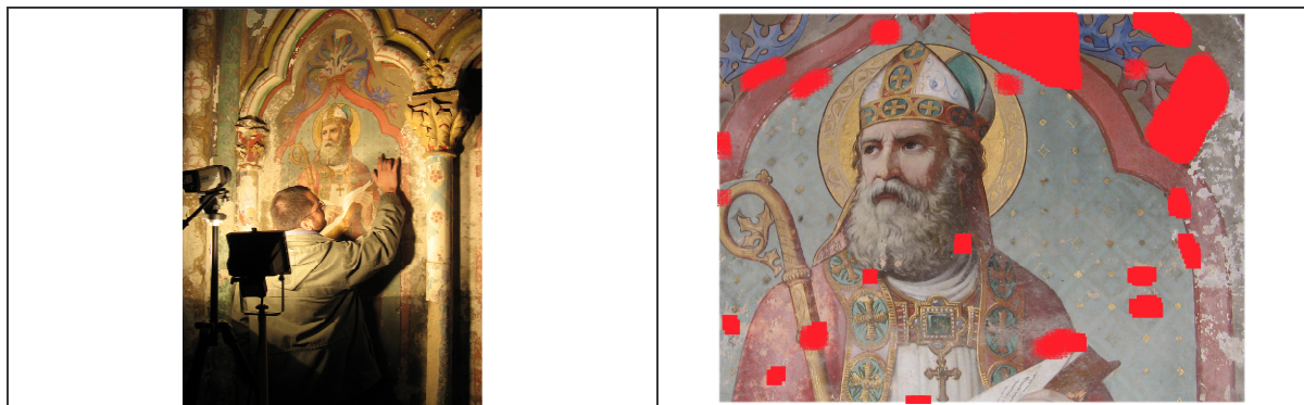
Fig. 10. Acoustic analysis of painting on canvas representing « Saint Martin » of the church of Bonnet
